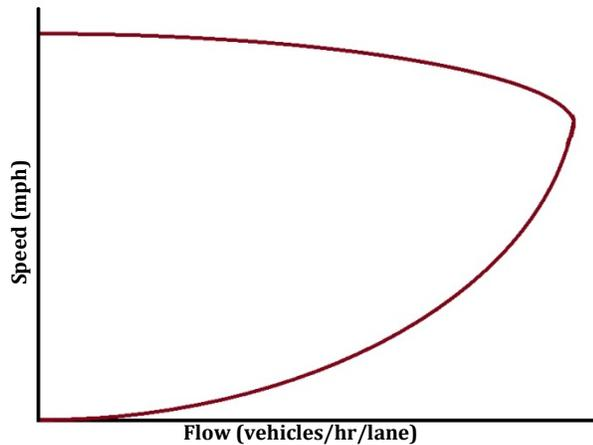
The diagram above shows the graphic relationship between traffic flow and speed. The purpose of using the variable speed limit technique is to slow traffic based on the flow before the characteristics pass the optimal point on the curve. Doing so can prevent the sudden decrease in speed and stop-and-go conditions commonly seen on congested roadways.
