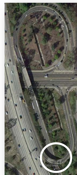
Partial Cloverleaf Interchange at State Route 170 and Roscoe Boulevard; Braided Loop Ramps at State Route 170 and Victory Boulevard. Aerial Photographs from Los Angeles, California. Source: Google Earth™
